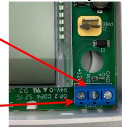
Wiring modification: No Change Needed Most coaches are wired using a 4/5-wire thermostat wire from the OE. For Dometic, only 3 wire leads are used. For Furrion, the 4th wire will need to be utilized.
